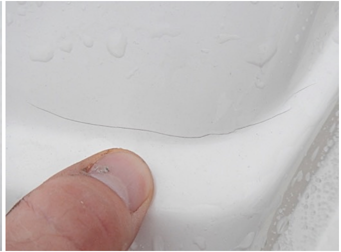
Gelcoat cracking at pilothouse windshield frame
