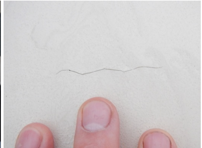
Gelcoat crack in foredeck non-skid
