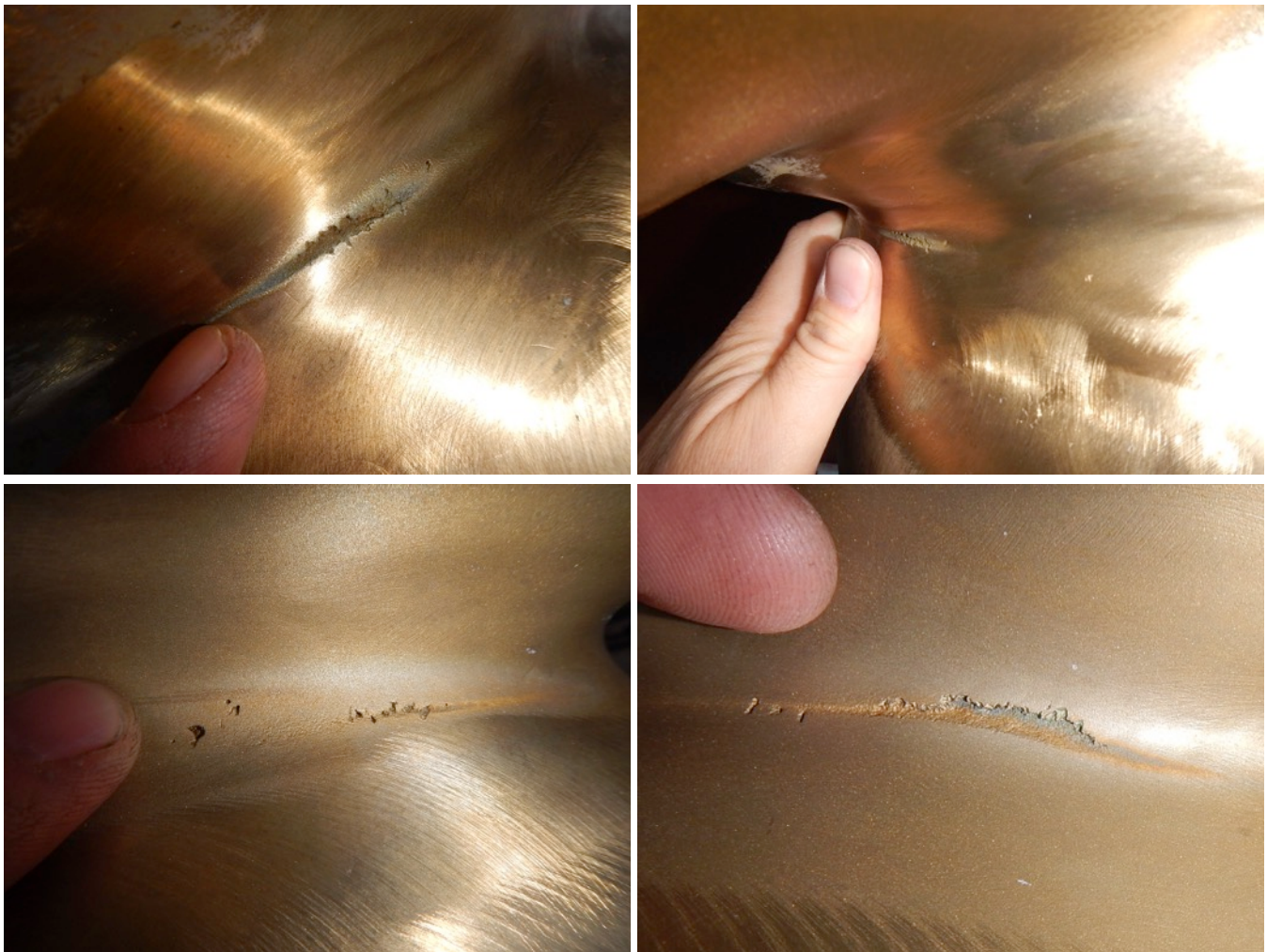
Erosion of bronze at prop hubs
