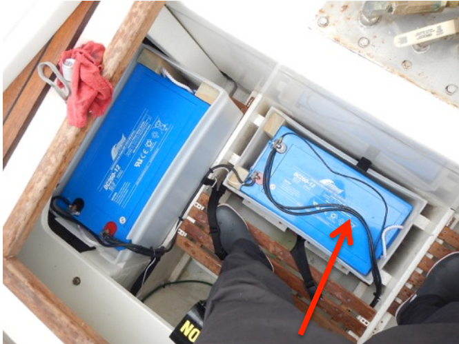
24V DC stern thruster power conductor is size #6 AWG
