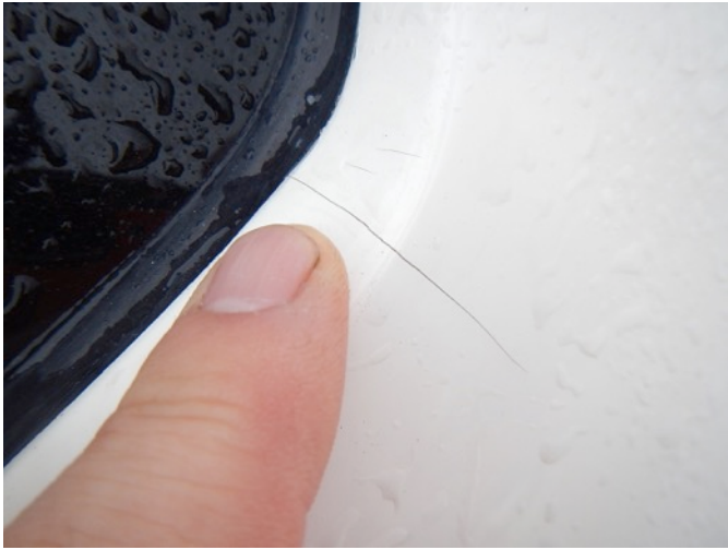
Gelcoat cracking at pilothouse windshield frame
