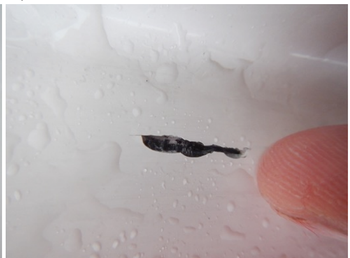
Gelcoat chip at air-bubble void
