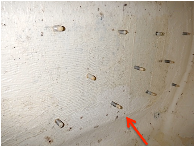
Bow pulpit fasteners not secured with nuts & backing washers
