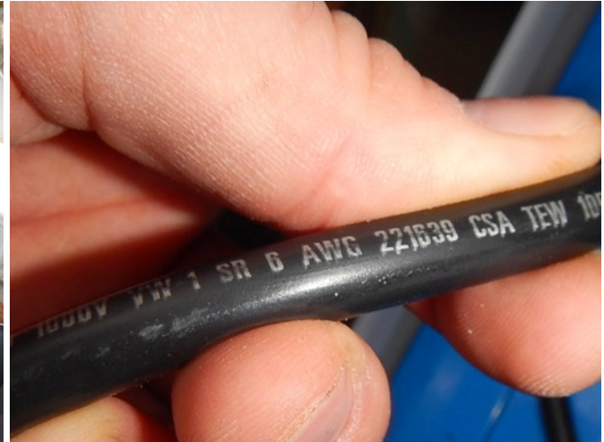
24V DC stern thruster power conductor is size #6 AWG
