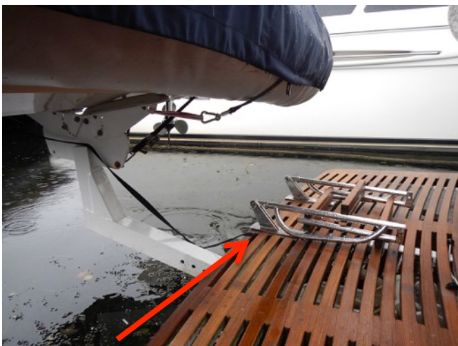
Reboarding ladder system is obstructed by the tender
