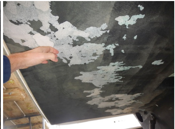
Bottom paint is deteriorating
