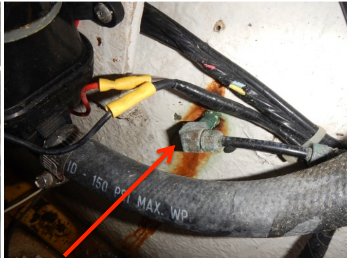
Water intrusion & crevice corrosion at trim tab cylinder fasteners
