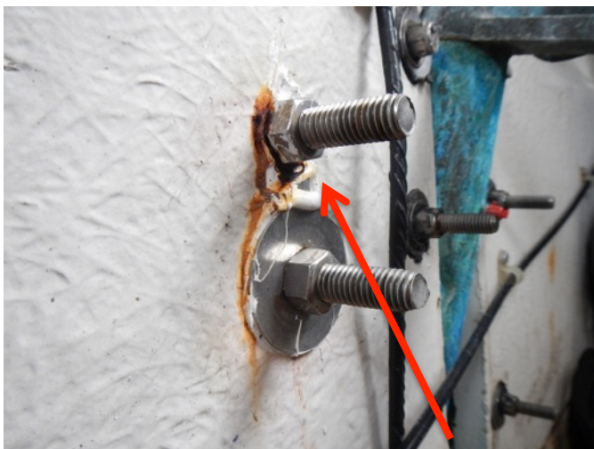
Water intrusion & crevice corrosion at U-bolt fittings
