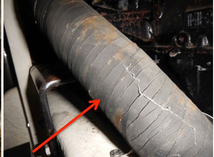
Main engine seawater intake hoses are cracking
