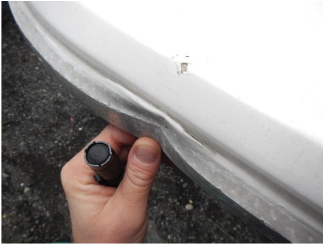
Dent in aluminum rub rail
