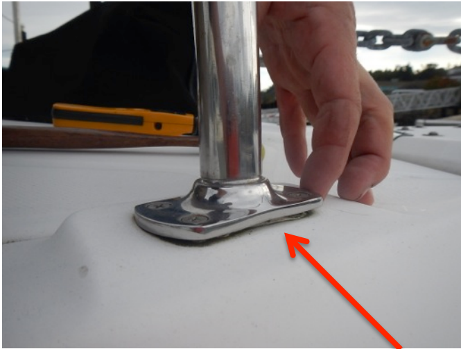
Bow rail stanchion base is loose. Fiberglass is damaged at stanchion base fasteners
