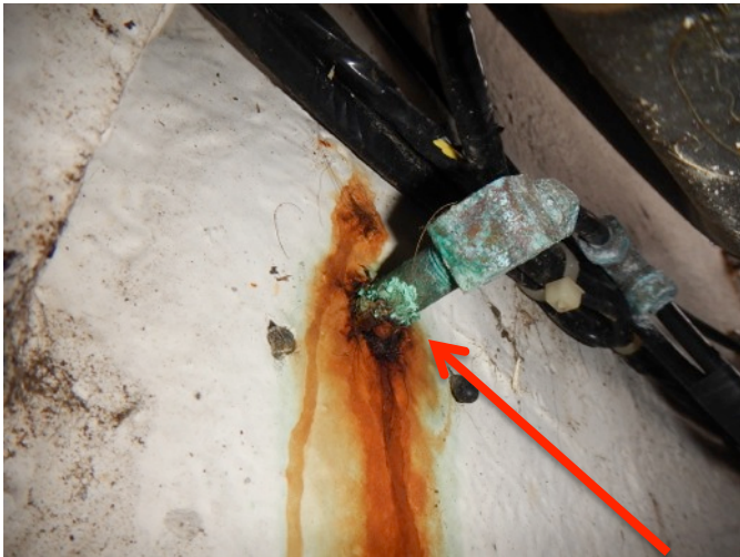
Water intrusion & crevice corrosion at trim tab cylinder fasteners
