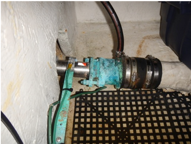
Starboard engine shaft seal leaking excessively
