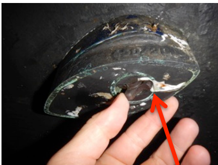
Paddle wheel is inoperable
