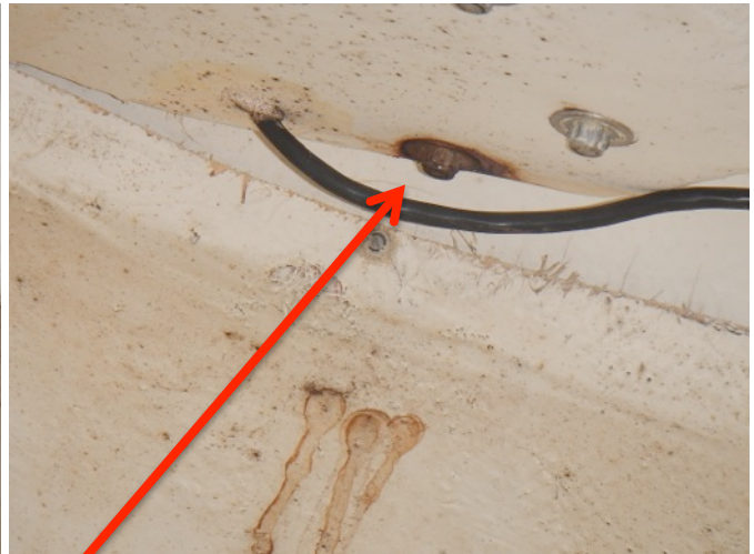
Water intrusion at pulpit structure fastener
