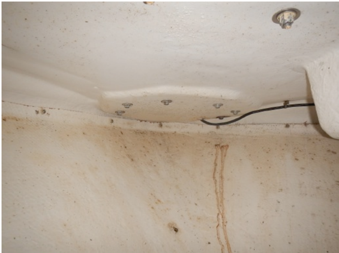
Water intrusion at pulpit structure fastener
