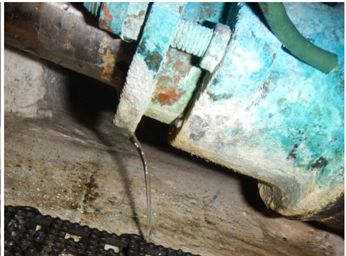
Starboard engine shaft seal leaking excessively
