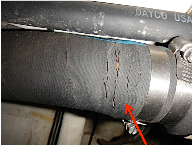
Main engine seawater intake hoses are cracking
