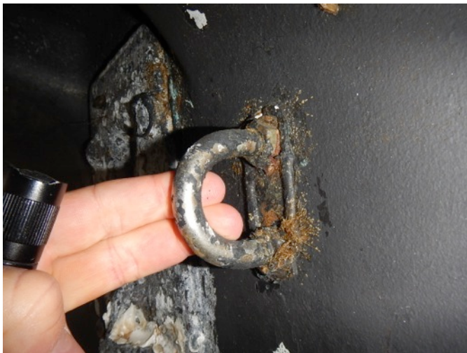
Zinc anodes are deteriorating
