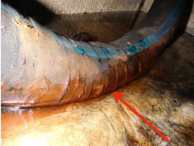
Main engine seawater intake hoses are cracking
