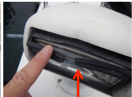
Search light is damaged
