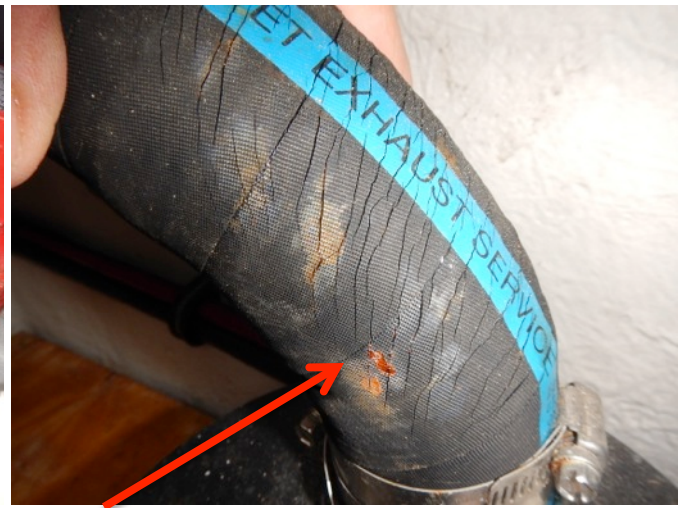
Generator exhaust hoses are cracking
