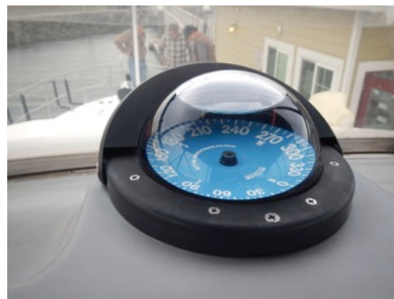
Air bubble in compass dome
