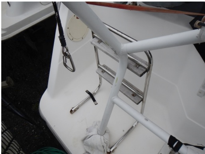
Reboarding ladder is obstructed by davit structure
